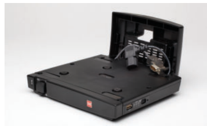
CodeManagement Module for use with LIFEPAK 20e Defibrillator/Monitor - Wireless Connects to the LIFEPAK 20e defibrillator to add wireless connectivity. 11150-000018
