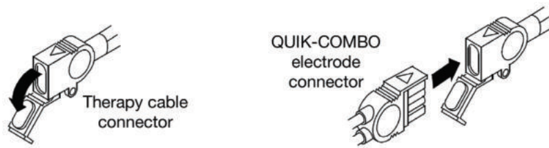
Figure 36 Connect QUIK-COMBO Electrodes to Therapy Cable
